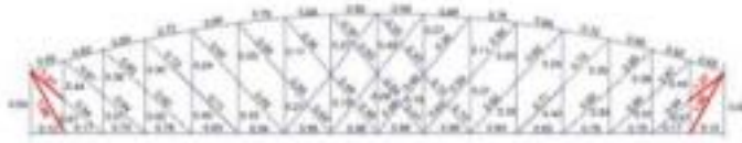
Fig. 7 Bridge steel member utilization in the arch base assuming a 15% corrosion allowance
